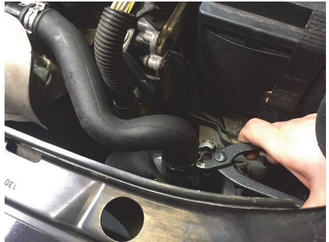
3. Remove the small clip under the intake and undo the 10mm bolt holding the airbox.
