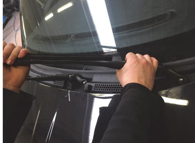
4. Remove the front of the cowl: first, remove the three clips using a screw driver.
