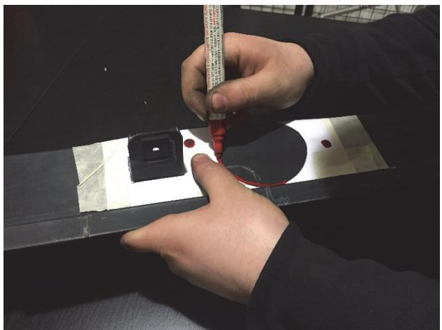
Cut and drill the holes out with a 7 mm drill-bit.
