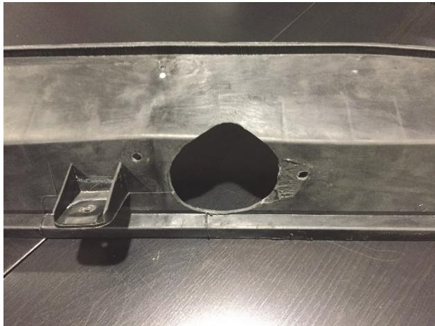
Rotate the panel 180° and remove milling the plastic rib shown below.
